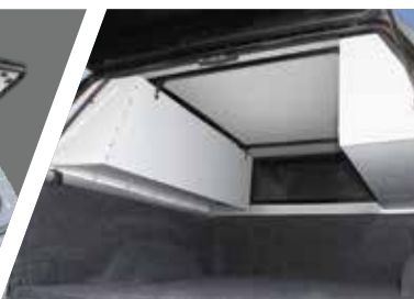
TOOLBOXES ARE SECURELY FASTENED TO ROOF FRAMEWORK
